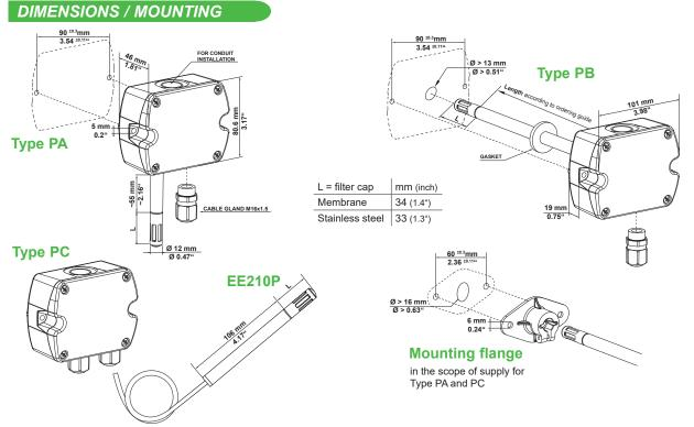
**EE210 with cable gland:** Use a matching wrench to install the cable gland (in the scope of supply) onto the EE210 enclosure. **EE210 with conduit connection** for the North American market: use a flat screwdriver to knock open the blind, carefully, in order to avoid damaging the electronics inside the enclosure. The conduit adapter is not included in the scope of supply. The M16x1.5 opening for the cable gland shall be tightly closed using the blind plug included in the scope of supply.
